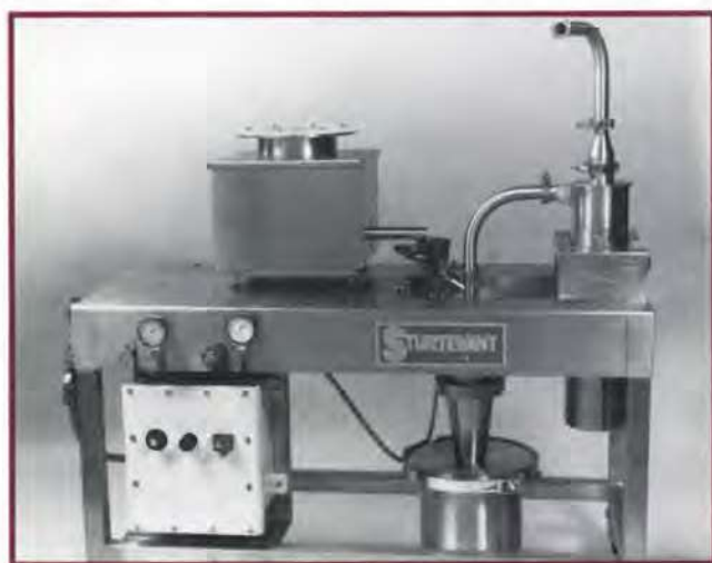
4" Micronizer, sanitary design, pharmaceutical grade, with primary and secondary cyclones and collection container.
